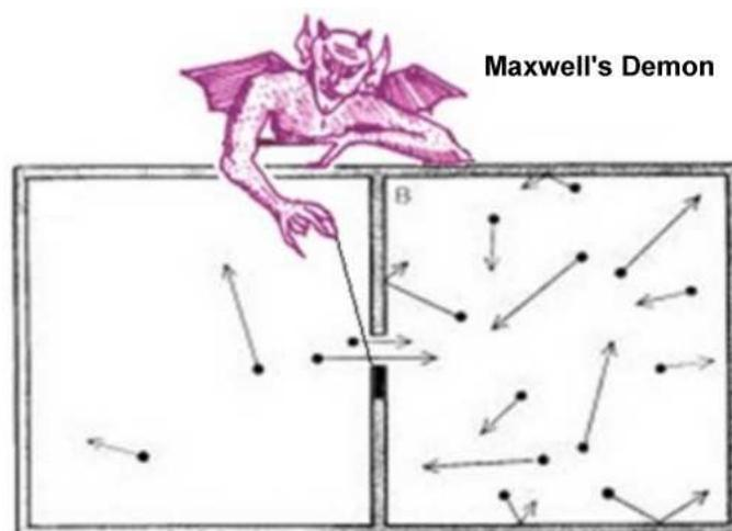
Take a container full of gas with a wall dividing it into two compartments. A small opening allows for communication between the two compartments, meaning that the gas is at the same pressure on
